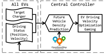
Fig. 7: System structure.
