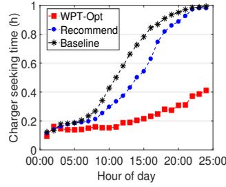
Fig. 10: Average charger seeking time of all EVs per hour.
