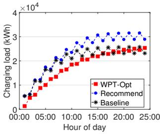
Fig. 13: Total charging load of all chargers per hour.
